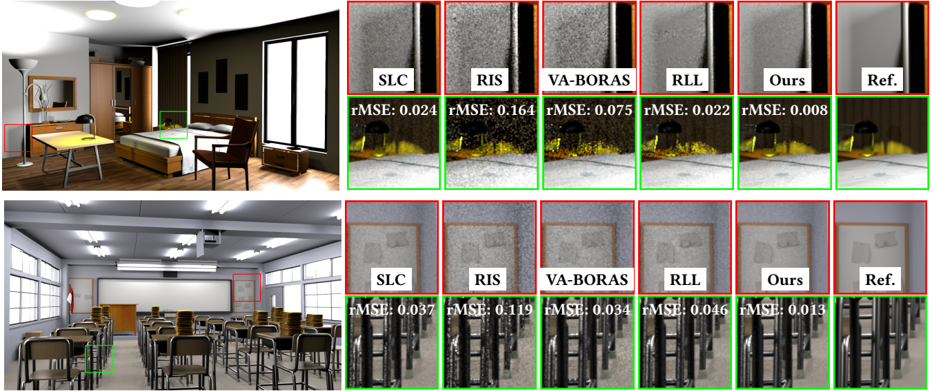
Fig. 4. BEDROOM and CLASSROOM. Equal-time comparison (120s) with SLC [Yuksel 2019], RIS [Bitterli et al. 2020; Talbot et al. 2005], VA-BORAS [Rath et al. 2020; Vévoda et al. 2018], RLL [Pantaleoni 2019] and our method. VA-BORAS does not cluster the lights properly. RLL produces stripe artifacts at the top row owing to its update rule. Our method is robust across different configurations and achieves lower error.
